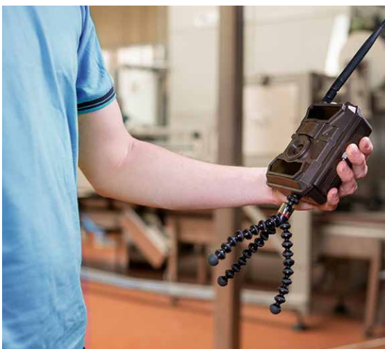
Pest Presence Surveillance camera with integrated SIM card. The camera can be placed (optionally with a trap or bait) in hard-to-reach locations with 24/7 surveillance for rodents
